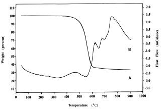
**Figure 1.** STA for polymer **5** under a nitrogen atmosphere at 10 K/min: (A) TGA curve; (B) DSC curve.
