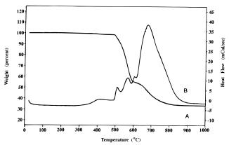
**Figure 2.** STA for polymer **5** under an air atmosphere at 10 K/min: (A) TGA curve; (B) DSC curve.
